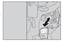
• When the staple cartridge for 65 sheets is installed, pull down the orange lever, and pull out the staple cartridge.
