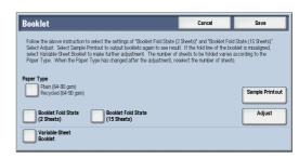
Select the state of the fold and staple position of the printout, and enter the 2-sheet stack misalignment amount you measured in step 6 in [Values A & B Before Adjustment].
