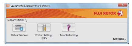
The Launcher window provides three buttons; Status Window, Printer Setting Utility, and Troubleshooting.
