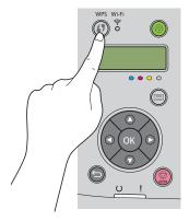
Start the WPS operation on the wireless LAN access point (Registrar) or router within two minutes.
