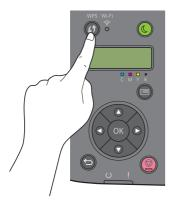
Start the WPS operation on the wireless LAN access point (Registrar) or router within two minutes.
