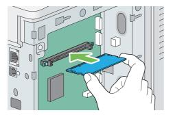
5 Push the memory module firmly into the slot.
