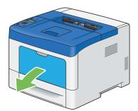
3 Grasp both sides of the bypass tray, and then pull the bypass tray from the printer.
