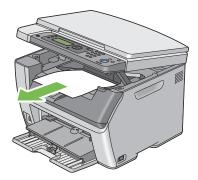
4 Remove any paper in the priority sheet inserter (PSI) or multipurpose feeder (MPF). Keep the paper wrapped and away from humidity and dirt.
