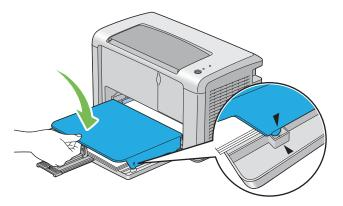
**10** Open the output tray extension by two steps. At the secondary step, extend it fully until it clicks.
