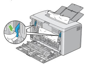
3 Remove any paper jammed from the back of the printer. If no paper is found in the paper path, then remove any paper jammed out of the center output tray.
