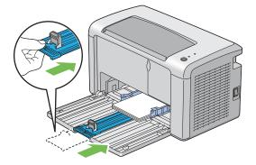
9 Insert the paper cover into the printer and then align the paper cover to the marking on the paper tray.
