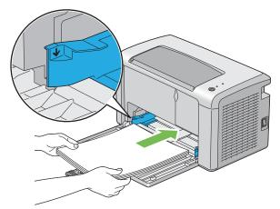
7 Adjust the paper width guides until they rest lightly against the edges of the stack of print media.
