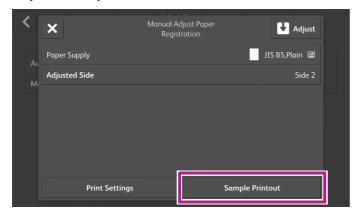
8. Confirm the printed sample, and input the adjustment values.
